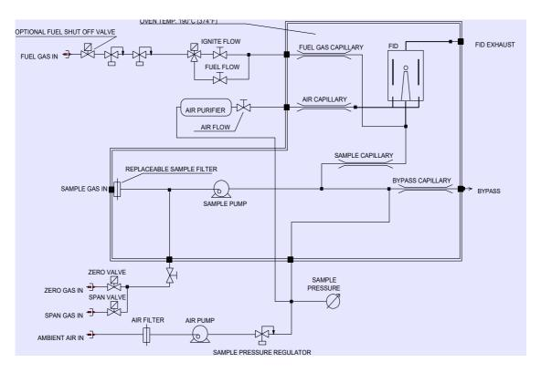
Complete flow diagram shown with alternative disposable sample filter Option OVE 7
