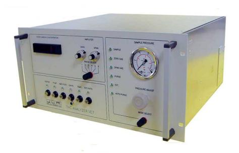
\*\*Low cost of ownership. \*\*Low fuel gas consumption. \*\*The combustion air supply for the FID-detector is built in. No external cylinder for synthetic air is needed. \*\*To prevent well known HC hang up (memory effect) and related drifting,the heated sample line can easily be connected inside of the heated oven. This prevents any cold spot and any related HC condensation.
